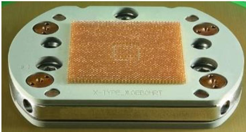
A wafer connector concept using traditional spring pins
